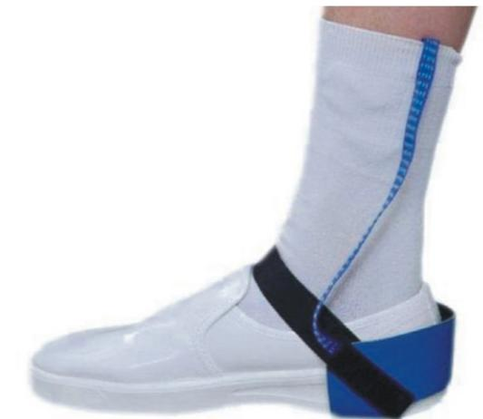
Consisting of conductive rubber, velcro and conductive weaving strap. Electricity will be discharged to conductive floor through conductive rubber. It is the best way to discharge the electro-static from human body. Earthing resistance:  $10^6 \Omega$
