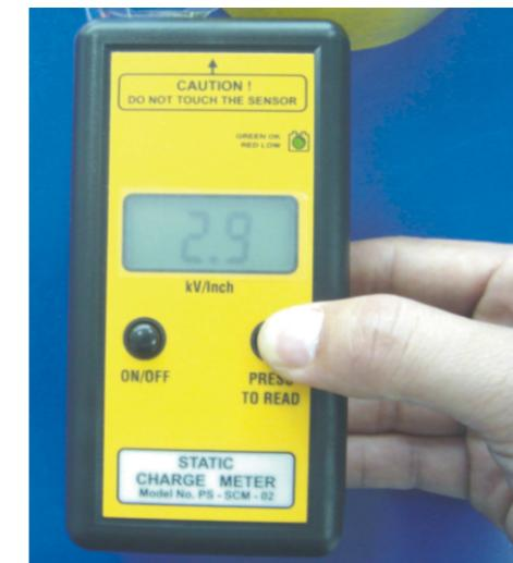
Reliable, highly accurate and low drift instrument for the measurement of magnitude static charges in terms of DC voltages. Easy to know whether any;
