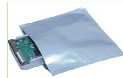
Its normal structure is ESD Polyester/Nylon / Aluminum / ESD Polyester. It has four main resistant function of static, electromagnetic interference and moisture proof. The product has superior puncture resistance and anti-static inner and outer layers with a surface resistance of  $10^8 - 10^{11} \Omega$ .
