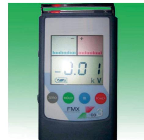
(Electrostatic field testing instrument) Simco FMX-003
